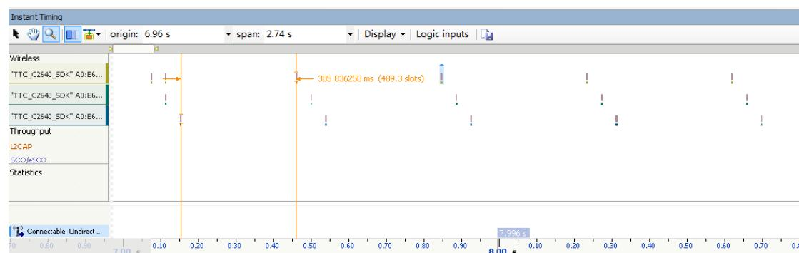
If the lower 4 bits are 1, multiple broadcasts are issued at the same time. "At the same time" means that there are 3 broadcasts in a short period of time. As shown below:
