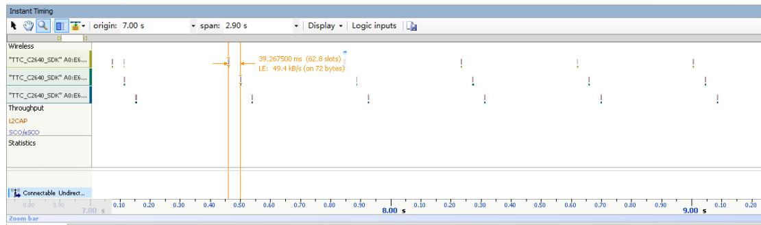
Example 2: Suppose you modify the Broadcast Mode register (0x17) by default to 0x30. The default broadcast interval is 300ms. High 4-bit value of 3, there are three broadcasts exist, as shown below is divided into three lines.
